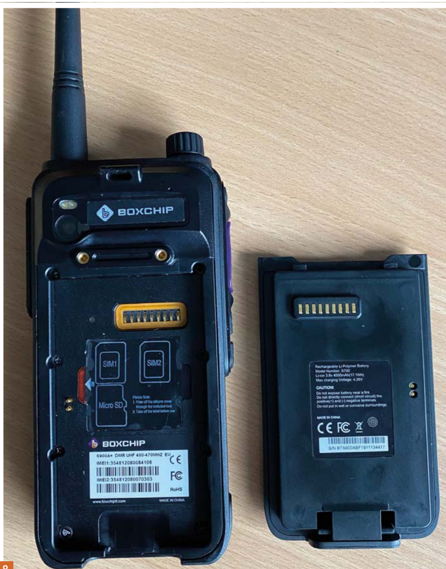
Fig. 4: The tiny microphone under the 'Back' button. Fig. 5: The left-hand side controls of the S900A. Fig. 6: There is a second microphone at the rear. Fig. 7: The right-hand side of the S900A, featuring the M6 port (and the dust cover). Fig. 8: The rear of the S900A, with a removable battery and dual SIM slots.
