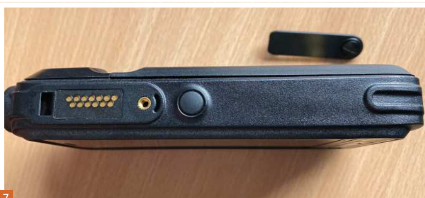
Fig. 4: The tiny microphone under the 'Back' button. Fig. 5: The left-hand side controls of the S900A. Fig. 6: There is a second microphone at the rear. Fig. 7: The right-hand side of the S900A, featuring the M6 port (and the dust cover). Fig. 8: The rear of the S900A, with a removable battery and dual SIM slots.
